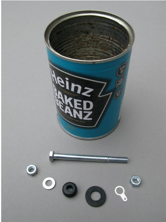
Fig. 3. Tin can (420 g) and bolt. Additional parts from left to right: M6 nut, M6 washer, 6.3 mm grommet (inside diameter), shower hose washer, M6 solder tag, M6 nut.
